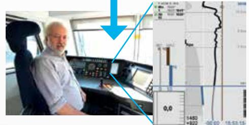
The standard CATO driver machine interface (CDMI) is ergonomic and displays the optimal speed profile and other important operational information.
